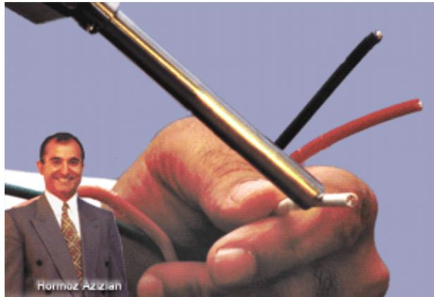
A fibre optic probe carrying near infrared light is placed on a wire insulation to scan and identify the plastic material.
