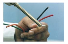
**Scanning time:** Normally, each measurement takes about 5 seconds and in most cases three to five measurements are taken for spectral averaging and identification purposes.
